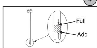
**NOTICE** Pause to permit oil to settle. Wipe dipstick clean each time oil level is checked. DO NOT overfill.
