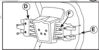
**NOTICE** By loosening both knobs to the unthreaded middle section of the attachment bolt, the upper handle can fold forward to store flat atop the cold engine. DO NOT fold the handle down while the engine is hot.
